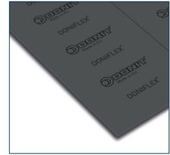
DONIFLEX® G-EM is an advanced composite material based on graphite and aramid manufactured under organic solvent-free conditions. DONIFLEX® G-EM is reinforced with expanded galvanized steel sheet insert. Even surface pressure distribution on gasket provides excellent thermo-mechanical properties and very good sealing characteristics. Therefore material is particularly suitable for petrochemicals, high temperature applications and valves.
